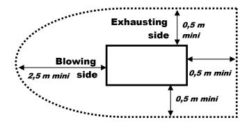
Do not to install the Heat pump in a confined place (the fan would recycle its air and the Heat pump would be down performance).
