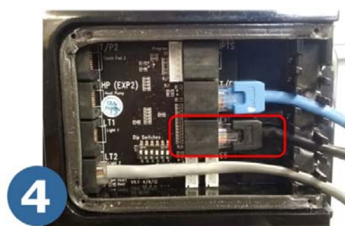
4 Connect black data cable from SmartSTREAM module into EXP1 socket
