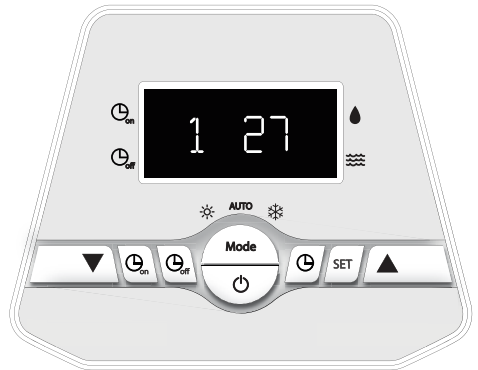
Parameter 1: Heating setting water temperature (10-45°C). Factory setting: 27°C
